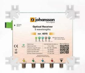
The **Optical Quintuple Receiver** is developed for the transmission of broadband signals in medium and large Fiber Optic systems. Ref. 4015 converts 1310 + 1330 + 1350 + 1370 + 1550 nm to  $2 \times V/H$  and CATV signal.
