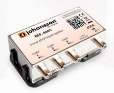
Standard **splitters** can give collisions when two commands come at the same time or when one of the set-top boxes uses a permanent high voltage. A smart splitter captures the commands of the different set-top boxes and serializes them to guarantee no collisions happen.
